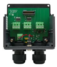
P/N 9203-2031082 AeroMate front cover assembly and counter module shown disassembled. Front cover assembly, shown with wireless kit, is easily removed for routine sensor maintenance.
