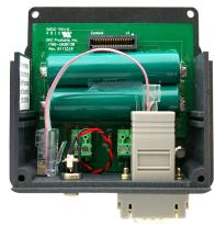
P/N 9203-2031090 AeroMate front cover assembly and uplink manager module shown disassembled. Front cover assembly, shown with wireless kit, is easily removed for routine sensor maintenance.
