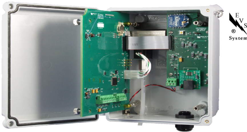
P/N 0928-2081000 PumpMate™ 2010 shown with optional 1-Valve control and wireless communication module.
