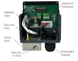
The 1x Valve includes one, dual-port, latching solenoid valve, 1/4-NPT female gas in port, 1/4-NPT female gas out port, an external power jack receptacle, a universal 2" pipe or motor valve mount, a 1/2" watertight bushing and rear panel gasket. Manifold material is 316 SS.
